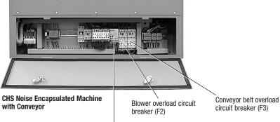
Motor overload circuit breaker (F1)
